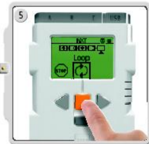
Now select if you want the program to Loop. This means that the program will run again and again until you switch off the NXT. For our little test, select Loop.
