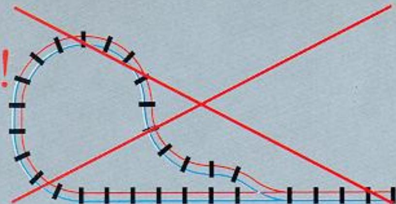
**UK** Short circuiting will result from some lay-outs of the 9V railway tracks, e.g. those shown here. If the track has short circuited, the green lamp on the speed regulator will be off, or very weak, and the train will not run. You can check for short circuiting of your track lay-out by allowing two different colours to follow the outer and inner rails. The track will short circuit if the two colours meet on the same side.
